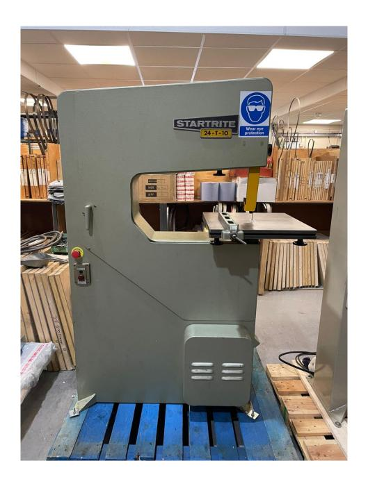
Variable speed industrial bandsaw for use on most materials.
