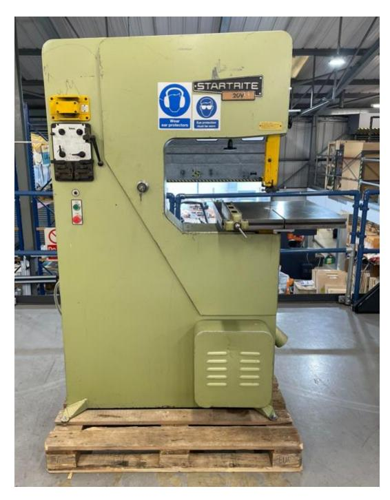
Variable speed industrial bandsaw for use on stainless steels right through to plastics or aluminium.
