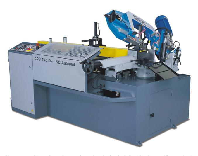
**Features and Functions:** The maximum length of a single feed is 500 mm. The required workpiece length is easily set with a hand lever and displayed on the digital meter. The Alligator 240 CNC is equipped with a more powerful motor and a frequency changer allowing for setting optimum saw blade speed between 25 and 100 m/mi. The optimum setting of saw blade speed towards the workpiece increases the productivity of the machine and the saw blade life.
